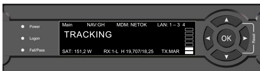
Figure 4-1: ACU: LEDs, display and keypad (detailed, example)
