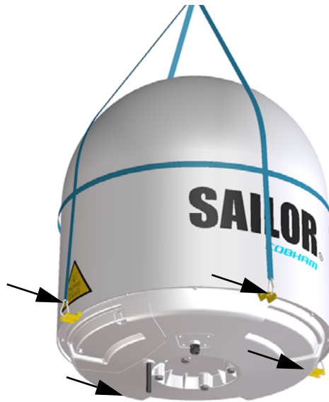
Figure 3-16: ADU installation, webbed sling attached to the 4 lifting brackets
